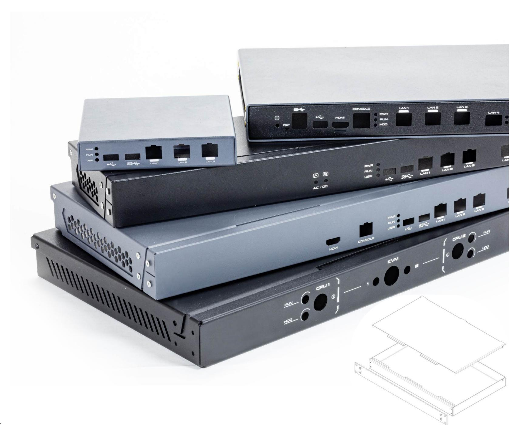
One of the block chassis options is a 19"-chassis especially designed for horizontal board insertion and non-standard component installation like transformers and other heavy-load accessories that are usually mounted on a support panel. REZOLUT offers sheet steel chassis (aluzink coated) with 3 mm-aluminum profile front panel, customer-configured, as well as aluminum chassis.
